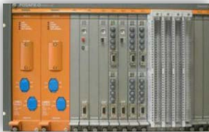
PLC (Programmable Logic Controller)
